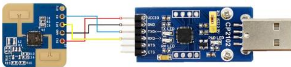
Figure 4-1 The connection method between HLK-LD2420 hardware and USB serial port adapter board
