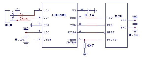
The image above is a reference circuit for one-key download of a multi-mode MCU based on USB to serial port, without manual setting or manual reset.
