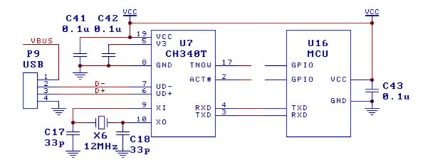
The image above is a sample design to achieve USB connection on an MCU by connecting it to a CH340 via TTL serial port. Here we use self-power mode, VCC supports 5V or 3.3V (V3 shorted to VCC if VCC is 3.3V), and don't use USB bus power VBUS at all (Can be tested by connecting series resistor to I/O of MCU if needed). CH340 shares the same power source with MCU, hence there would be no current inrush through I/O between CH340 and MCU.
