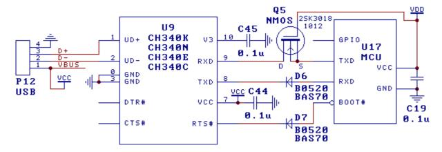
The image above is a sample design to achieve USB connection on an MCU by connecting it to a CH340 via TTL serial port. CH340 is powered by USB bus VBUS. MCU is powered by another power source VDD, VDD supports 5V, 3.3V and even 2.5V, 1.8V.
