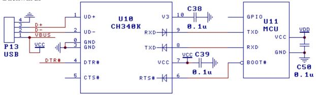
The figure above shows the reference circuit of MCU connecting CH340K chip through TTL serial port to realize USB communication under dual power supply mode. The CH340K is powered by the USB bus, VBUS (VCC), and the MCU uses another power supply VDD, which supports 5V, 3.3V or even 2.5V and 1.8V. The backplane of CH340K package is an optional GND pin, which can be easily connected to GND or suspended according to PCB routing.
